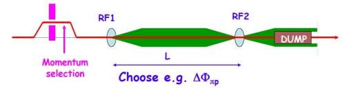
Particle species separation by radio-frequency modulation
