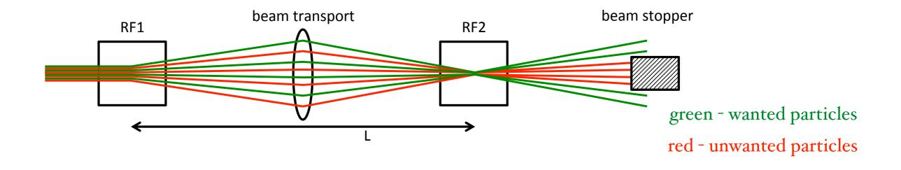
Momentum limits with current technologies due to the length (1.1 km) of the M2 beam line: kaon beam  $\sim 75 \ GeV/c$ anti-proton beam  $\sim 108 \ GeV/c$
