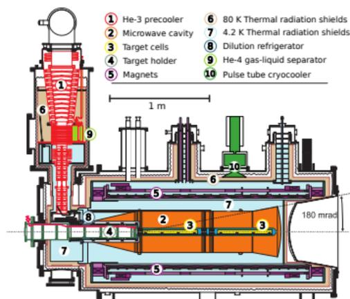
Polarised target cryostat.
