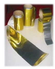
Long flat aluminium-polyimide multilayer flexible buses (thickness < 50  $\mu$ m) Technology in Ukraine (microcable production and micro electronics assembly) used in numerous experiments
