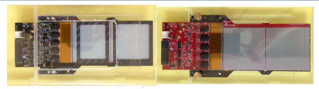
The Silicon detector unit developed for BM@N experiment at NICA. The unit contains electronics for 640 strips. The front-end electronics is based on a charge sensitive preamplifier chip VATAGP7 (IDEAS)
