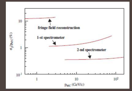
The relative error  $\sigma p/p$  is about 0.5% for tracks reconstructed in both spectrometers (p >= 5 GeV/c) and about 1.2% for low momentum tracks reconstructed in the LAS only.
