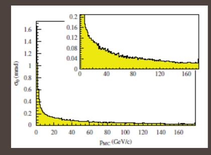
The error on the track polar angle at the interaction vertex ( $\sigma_{\theta}$ ) is of the order of 0.1 mrad for p about 30 GeV and increases for lower momenta
