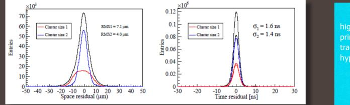
high resolution of the primary vertex position and tracking to reject pbar from hyperons decay  $(\Lambda, \Sigma)$
