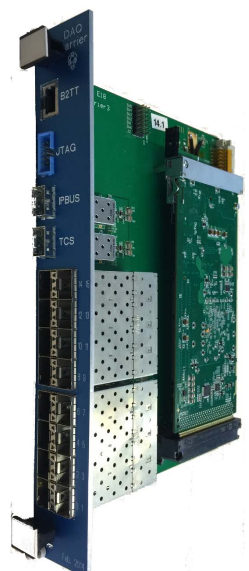
DHC on VME carrier Card as used for DHCmx and DHCsw
