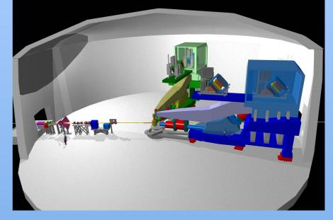
Spectrometer Pair, polarized <sup>3</sup>He target up to to 10<sup>38</sup> cm<sup>-2</sup> s<sup>-1</sup> hadron ID
