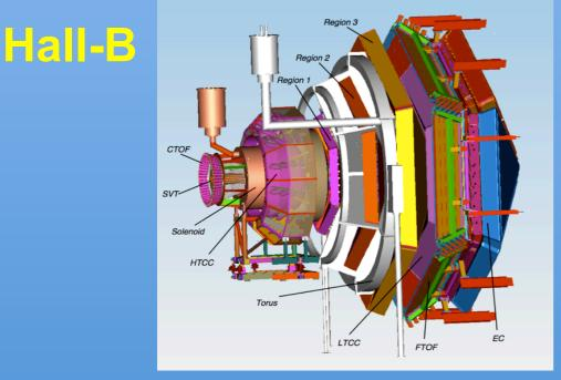
CLAS12 H,D polarized targets up to 10<sup>35</sup> cm<sup>-2</sup> s<sup>-1</sup> "complete" acceptance, hadron ID
