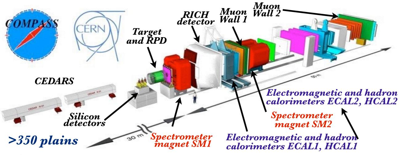
CEDAR detectors for beam particle identification
