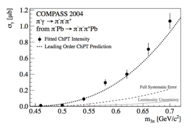
COMPASS already published the result for the cross section of  $\pi^-\gamma \rightarrow \pi^-\pi^+\pi^-$  reaction near threshold.
