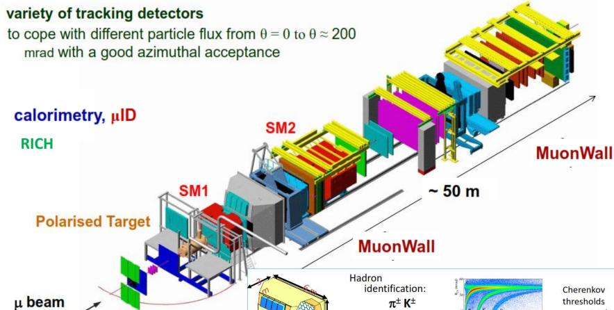
Cherenkov thresholds  $\pi \sim 3$  GeV/c K  $\sim 9$  GeV/c p  $\sim 18$  GeV/c
