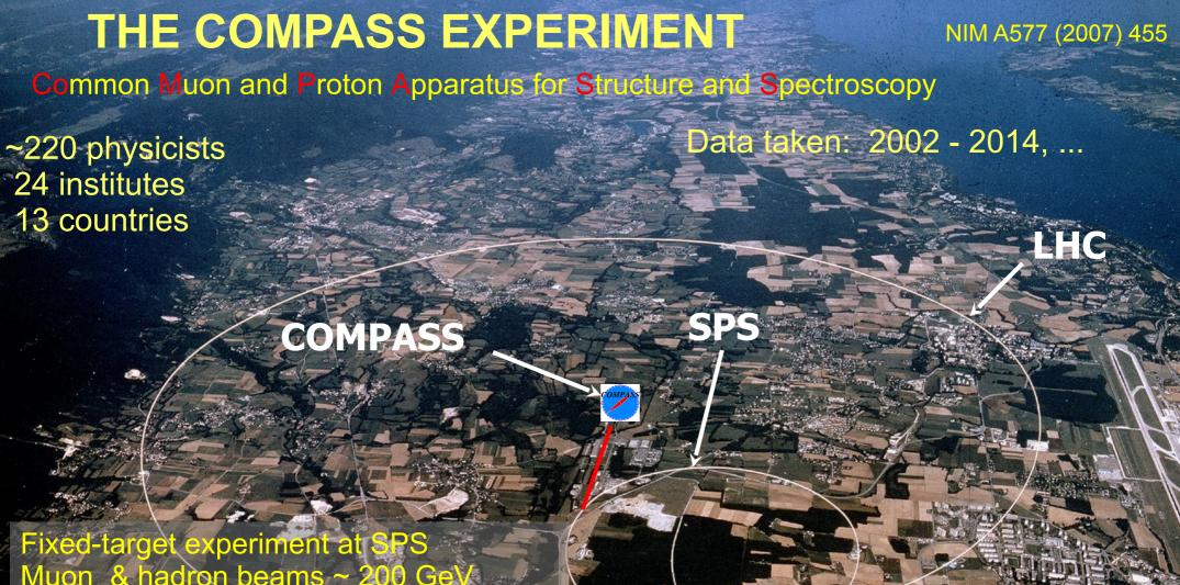
Muon & hadron beams ~ 200 GeV Polarised p&d targets Versatile spectrometer Running since 2002 Nucleon structure & hadron spectroscop
