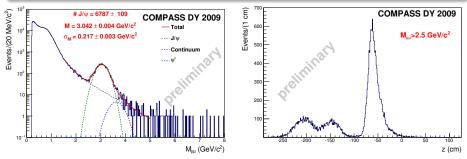
•  $J/\psi$  yealds confirmed,  $M_{J/\psi}$  and  $\sigma_M$  in agreement with the MC simulation. • target cells and beam plug distinguishable, better  $Z_{vtx}$  resolution with the new absorber and the vertex detector.
