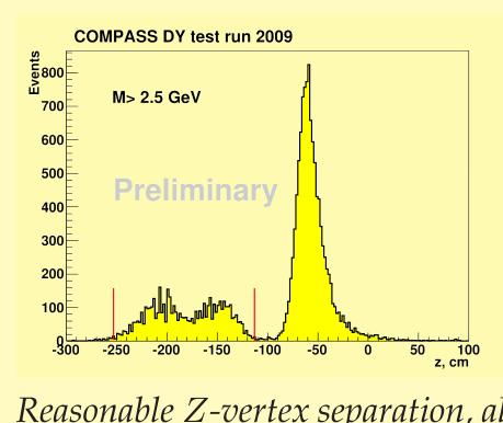
Reasonable Z-vertex separation, allowing to distinguish the 2 target cells and the absorber.
