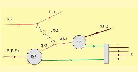
In single polarised Drell-Yan (DY), with transversely polarised target nucleons, the expression of the cross-section at leading order is [S. Arnold, et al, Phys.Rev. D79 (2009) 034004]:
