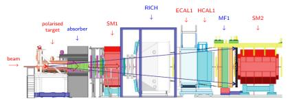
View of the COMPASS Large Angle Spectrometer from CAD design
