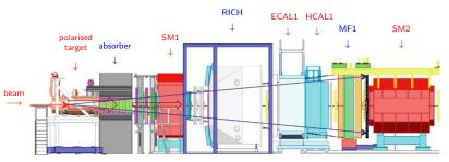
View of the COMPASS Large Angle Spectrometer from CAD design
