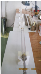
Prototype of the 2.5m long LH 2 target + test of the cryostat
