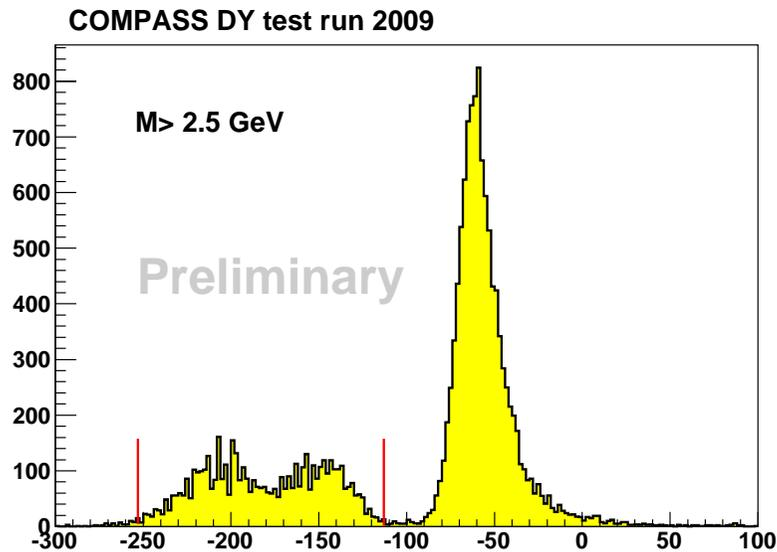
Reasonable  $Z_{vertex}$  separation, allowing to distinguish the 2 target cells and the absorber.
