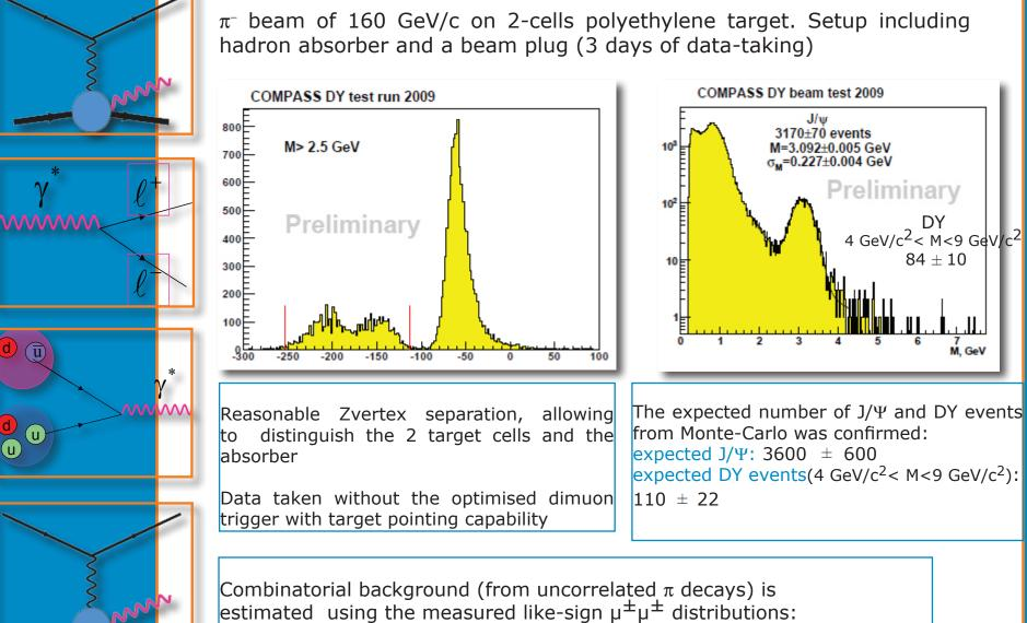
the absorber reduces the background by a factor 10 at  $M_{\mu\mu} = 2 \text{ GeV/c}^2$
