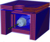
Structure of the absorber and its shielding
