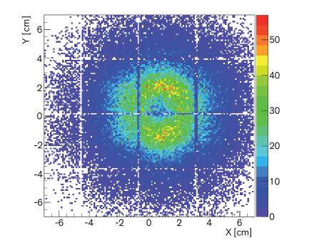
The largest fraction of Primakoff photons is deposited within 4×4 calorimeter blocks.
