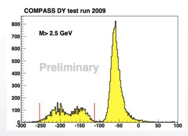
Reconstructed z-vertex position: two target cells and absorber are visible
