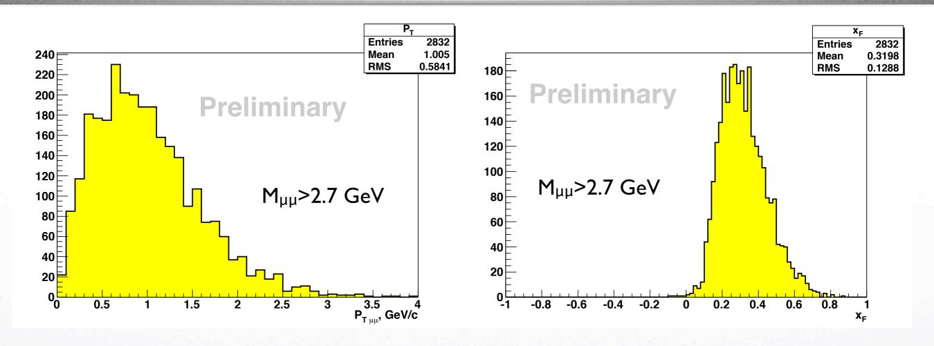
Kinematic distributions for  $x_f$  and  $p_T$  of dimuon obtained during Drell-Yan test run 2009 correspond to our expectations
