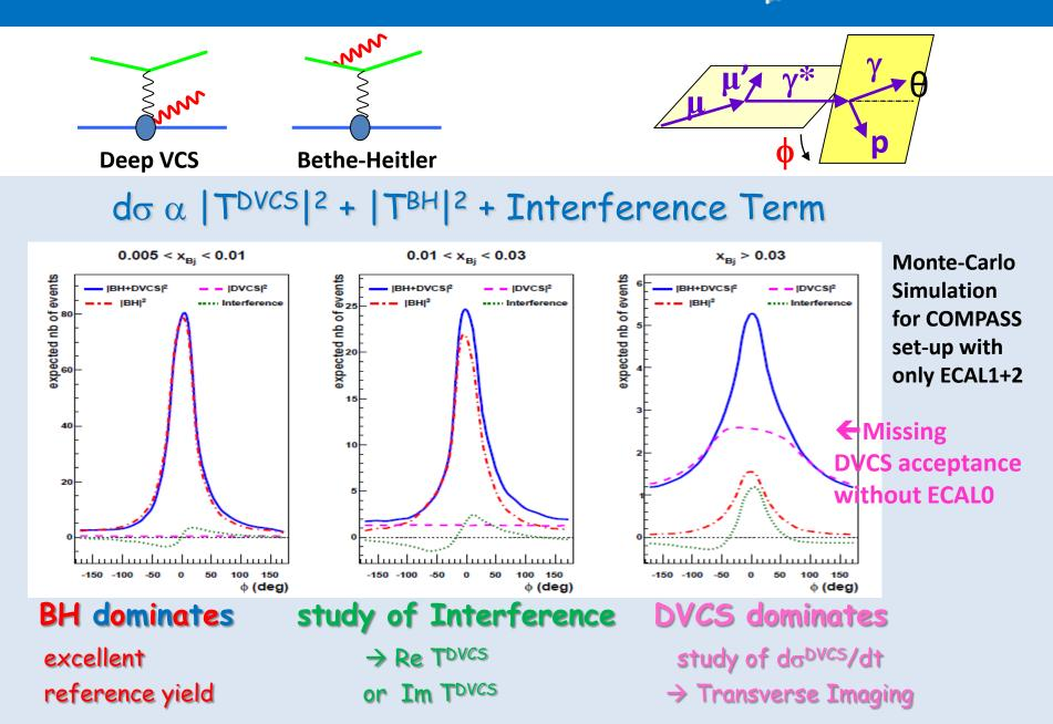
Projections for Phase 1 in COMPASS-II (2013-15) with recoil proton detection and hydrogen target
