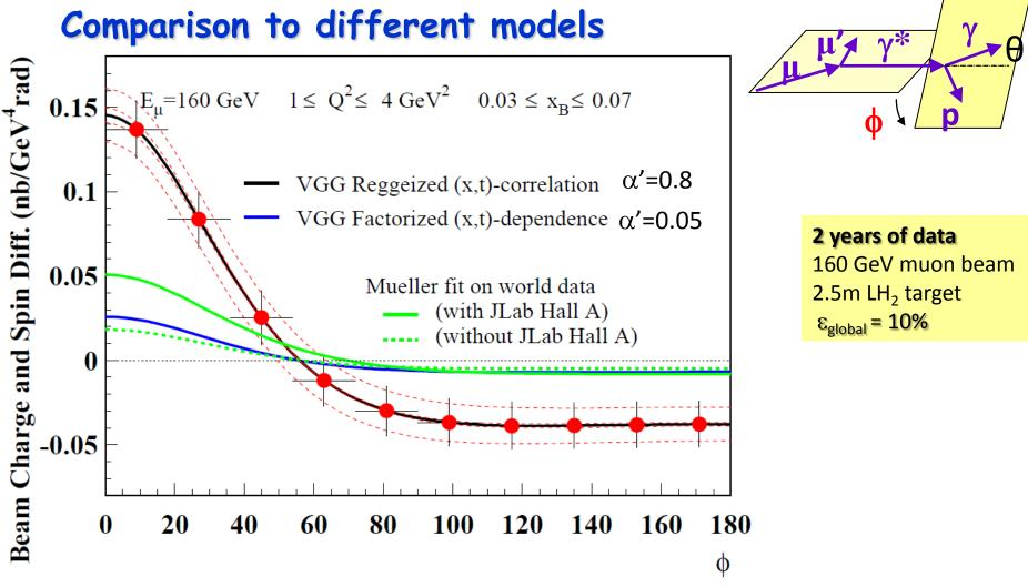
High precision beam flux and acceptance determination Systematic error bands assuming a 3% charge-dependent effect between  $\mu$ + and  $\mu$ - (control with inclusive evts, BH...)
