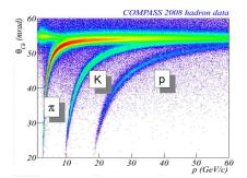
COMPASS's RICH detector allows separating Kaons from Pions up to some 30–40 GeV via measurement of particle velocity. Used here to identify final-state charged Kaons.
