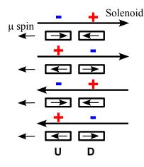
"+" – when direction of target cell polarization, coincide with direction of muon beam polarization.
