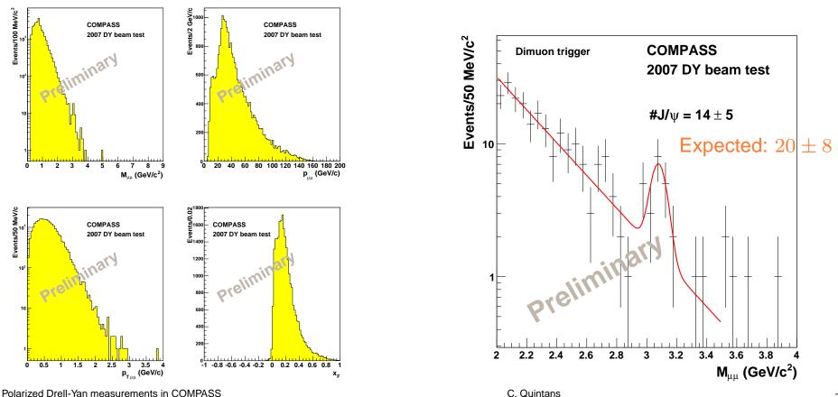
In 2008, a test without hadron absorber and increasing the  $\pi^-$  beam intensity was done  $\hookrightarrow$  even at 1/4 of the proposed beam intensity, we observe too large detectors occupancy.
