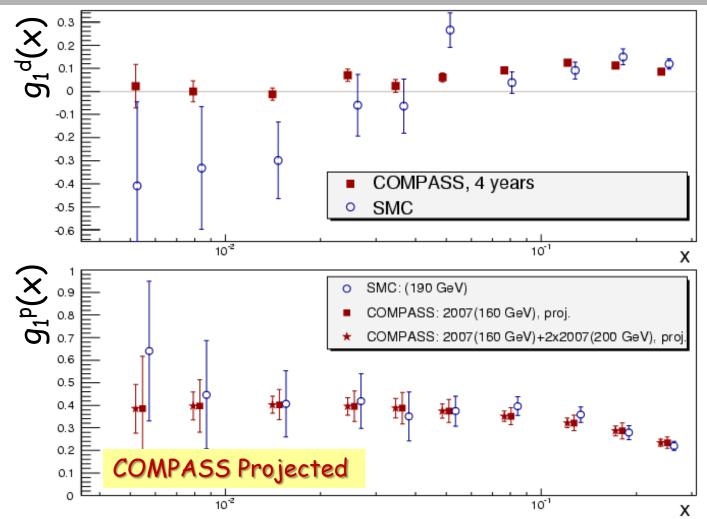
Figure 3: The spin-dependent structure function of deuteron  $g_1^d(x)$  and of proton  $g_1^p(x)$ . For comparison COMPASS points are shown together with SMC measurements. The  $g_1^d$ points (top) correspond to full deuteron statistics. For  $g_1^p$  (bottom), values are derived from the DSSV [13] polarised PDFs and the errors correspond to the statistics of 2007 and to the total statistics expected after another year of data taking.
