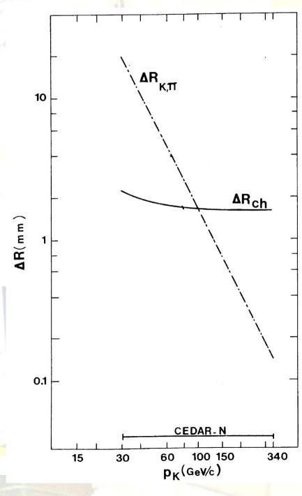
$R(\lambda) = f \cdot \Theta(\lambda) = \arccos\left(\frac{1}{n(\lambda)\beta}\right)$ spectral range of PMTs:  $\Rightarrow \Delta R_{ch} = R(500 \text{nm}) - R(200 \text{nm})$
