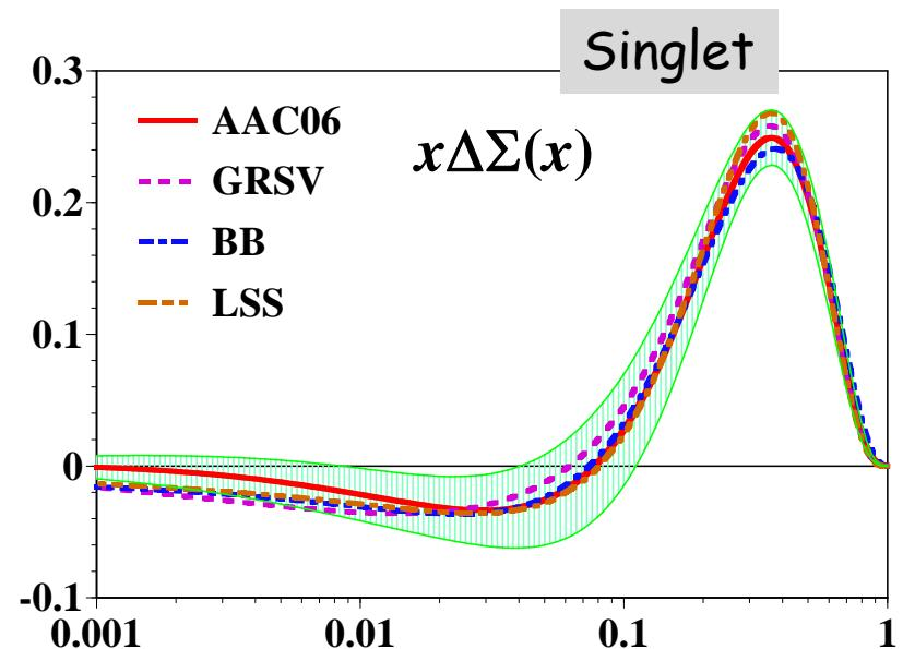
note: errors of AAC account for simultaneous deviation of all parameters
