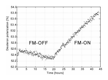
This plot shows the build-up of deuteron polarization in LiD over time with and without FM
