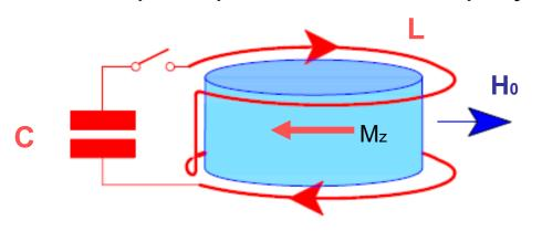
resonant circuit, tuned on the nuclear Larmor frequency, has no losses.
