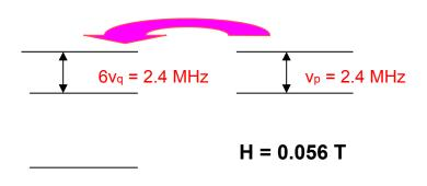
In 0.056 T field N<sub>14</sub>-quadrupole and Zeeman proton splitting are equalized and the fast cross-polarization between N<sub>14</sub> and 1H enlarged N<sub>14</sub> polarization from 14 to 50 %.
