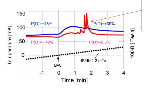
Here you can see the coherent radiation of D and Li<sub>7</sub> obtained on the COMPASS polarized target at CERN
