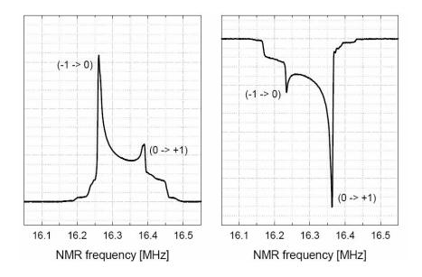
NMR-signals of D-propanediol (left) and D-butanol (right) with record polarizations of -81 % and +80 %, respectively
