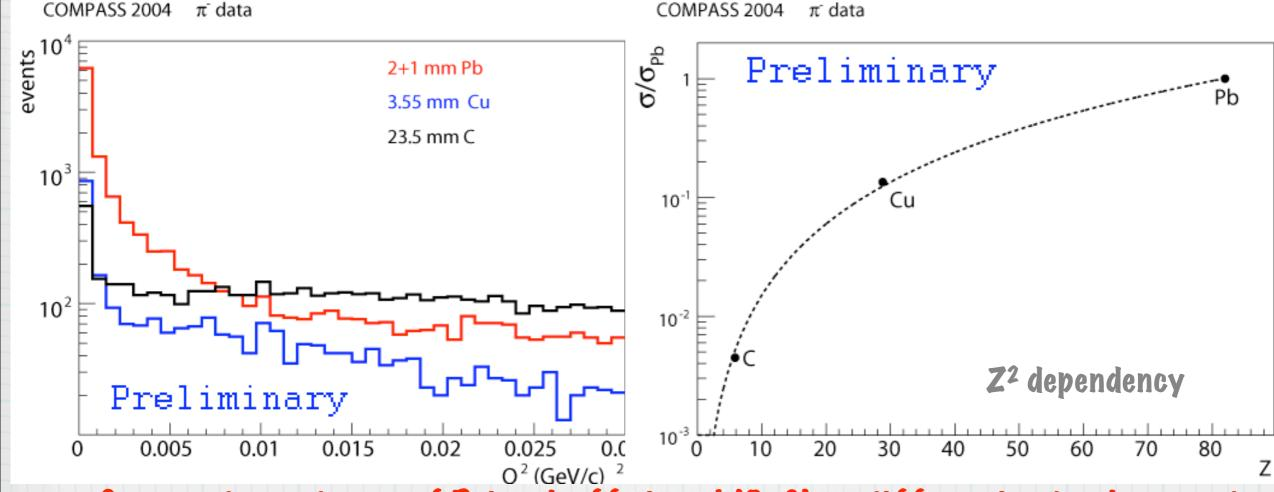
Strong dependency of Primakoff signal (Q=0) to diffractive background (Q>>0.01) ratio on the target material
