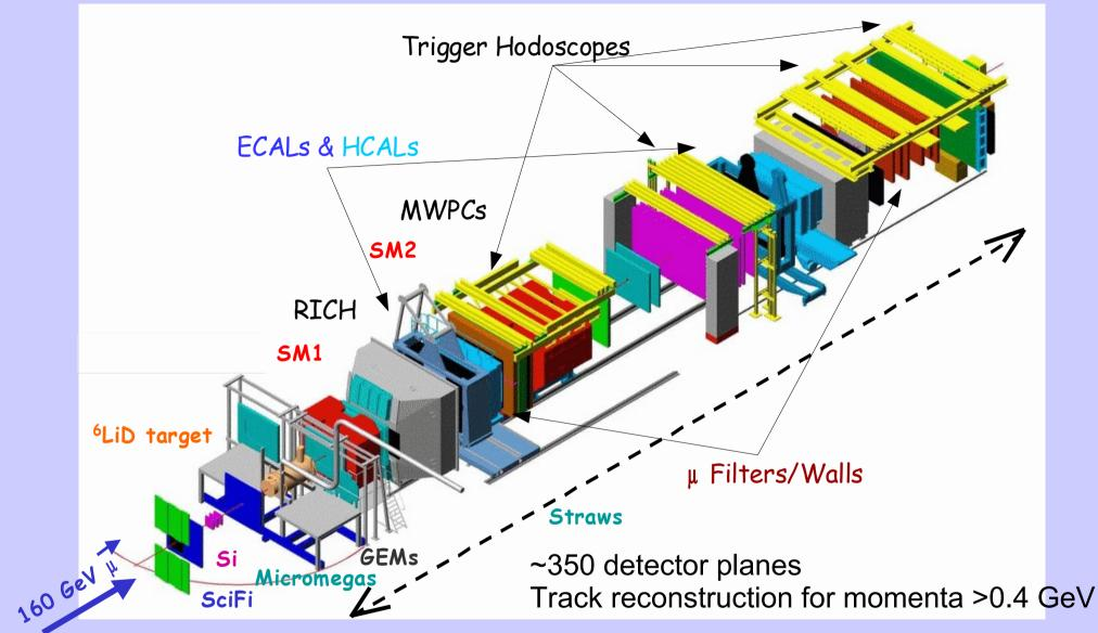
Two-stage forward-spectrometer: LAS – 1 Tm magnet (±180 mrad) SAS – 4.5 Tm magnet (±30 mrad)
