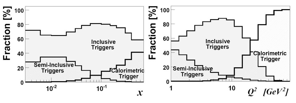
60—75% of inclusive triggers over the full COMPASS x range Semi-inclusive triggers dominant at low x and low Q<sup>2</sup> Calorimetric triggers dominant for Q<sup>2</sup> > 30 GeV<sup>2</sup>
