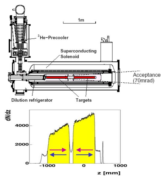
Two 60 cm long target cells with opposite polarisation Target material: <sup>6</sup>LiD Polarisation ~ 50% Solenoid field: 2.5 T  $^{3}$ He/ $^{4}$ He: T<sub>min</sub> ~ 50mK Field reversal every 8h
