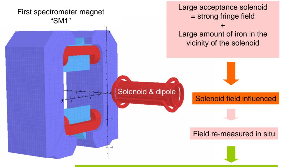
Correction coils settings for homogeneity <10<sup>-4</sup> over 130 cm
