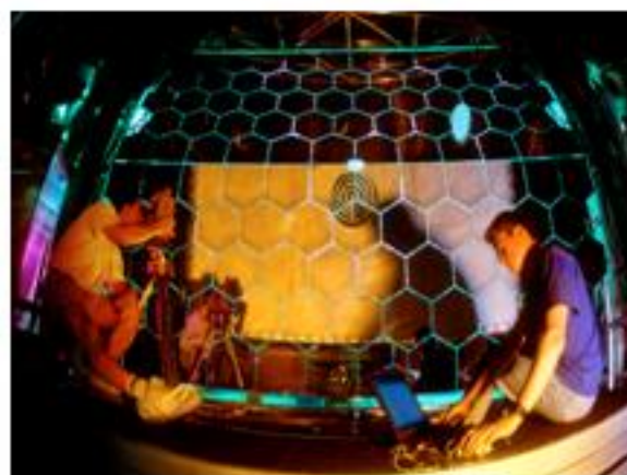
RICH CSl & MWPC readout Radiator: C 4 F 10
