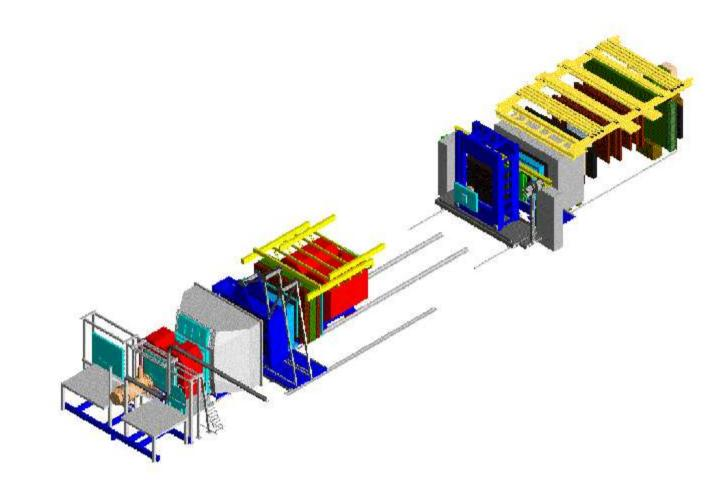
Naturally polarized  $\mu^+$  beam at 160 GeV/c ( $P_B \approx -76\%$ ) Beam intensity:  $2 \times 10^8 \ \mu^+$ /spill (4.8/16.2 s) Longitudinally polarized  $^6LiD$  target ( $P_T \approx 50\%$ )
