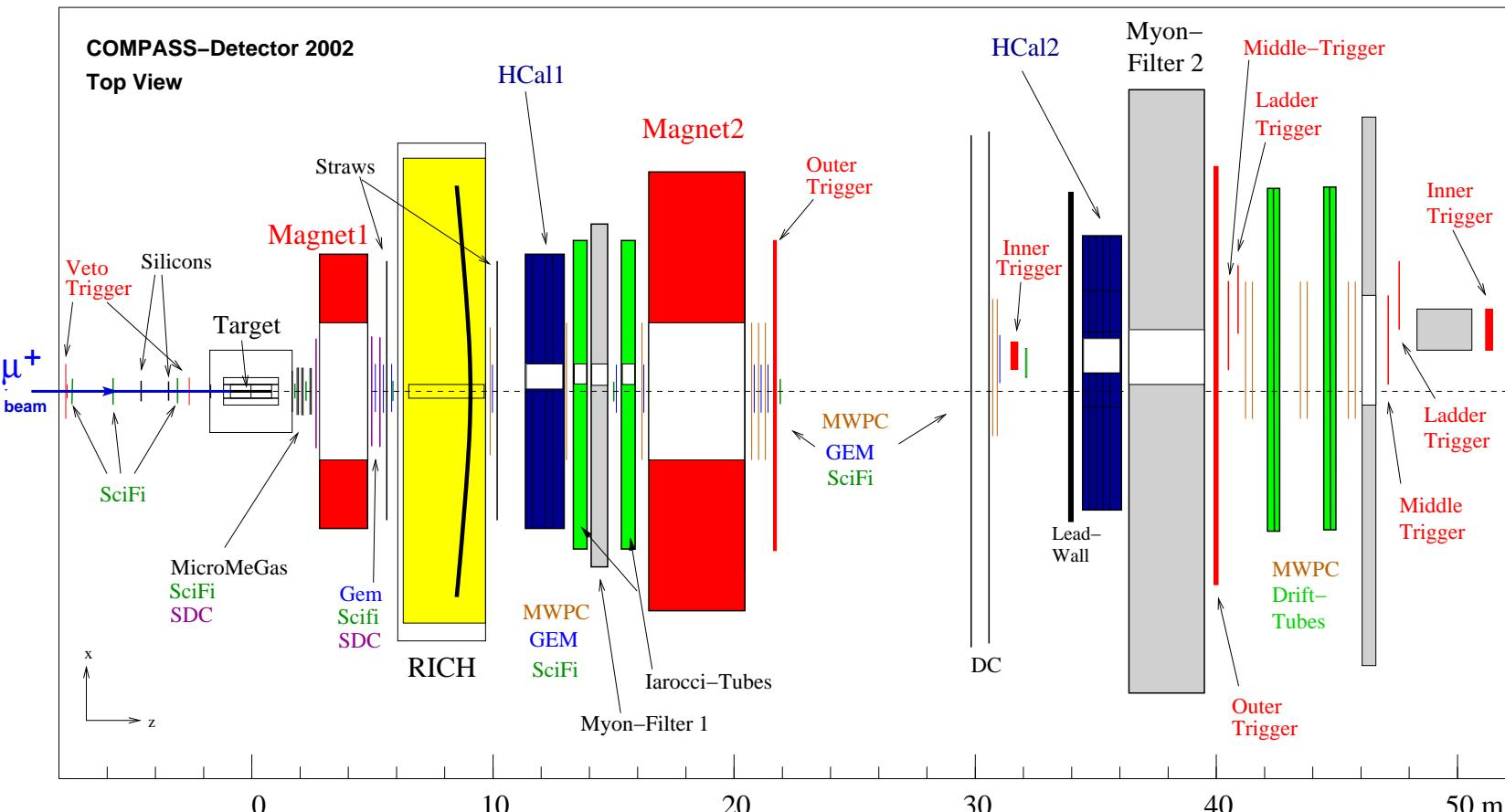
**Beam**  $2 \cdot 10^8 \mu^+/\text{spill}$  (4.8s / 16.2s)    **Beam momentum** 160 GeV/c
