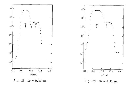
CEDAR-N pressure scan showing the  $\pi/K$  separation in the H6 beam running at -175 GeV/c.
