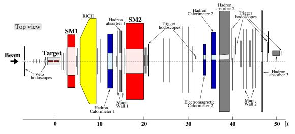
FIGURE 1. Layout of the COMPASS spectrometer in 2002 and 2003
