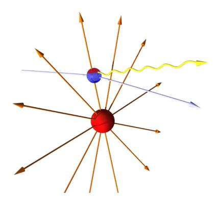
**Figure 1:** Visualization of the Primakoff Compton process: A high-energetic pion scatters in the electric field of a nucleus. For the magnetic contribution, it is to be realized that the nucleus passing the pion at high velocity represents an electric current inducing a magnetic field at the position of the pion.
