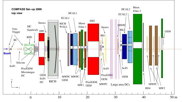
**Figure 2:** Layout of the COMPASS setup for hadron beam as used in the beam times of 2008 and 2009. A detailed description of the employed detectors is found e.g. in Reference [21]. The spectrometer magnets SM1 and SM2, surrounded by tracking detectors and followed by the calorimeters, constitute the two stages of the setup.
