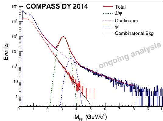
**Fig. 6**  $\mu^+\mu^-$  pair invariant mass spectrum from the 2014 Drell–Yan test run together with the measured combinatorial background from uncorrelated muons
