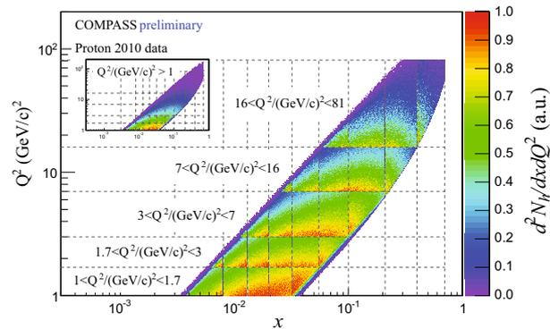
**Fig. 3** The  $x - Q^2$  grid which has been chosen to evaluate the transverse spin asymmetries. The region with  $Q^2 > 16$  (GeV/c)<sup>2</sup> is the so-called safe region for the Drell–Yan measurement
