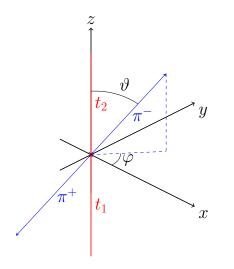
**Figure 5:** Definition of the decay angles
