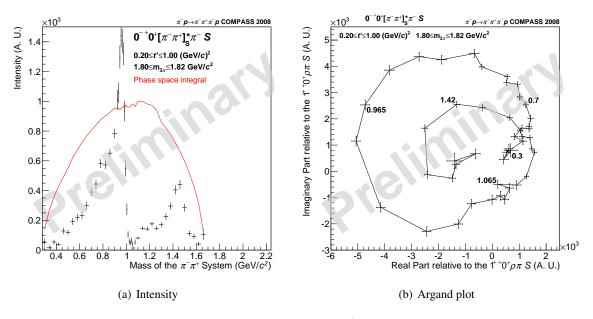
**Figure 12:**  $[\pi\pi]_S^*$  amplitude at  $m_{3\pi} = 1.80 \,\text{GeV}/c^2$  (white lines in Figure 11).
