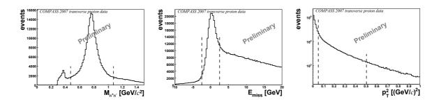
Figure 1: Distributions of  $M_{\pi\pi}$ ,  $E_{\text{miss}}$  and  $p_t^2$  for the NH<sub>3</sub> target with indicated cuts.
