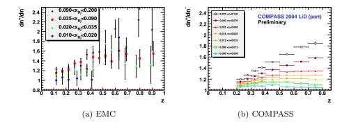
Fig. 2. Charged hadron multiplicity ratios  $dn^+/dn^-$  as function of z for EMC [5] and COMPASS.
