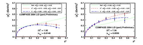
**Fig. 8.** Fitted  $\langle p_T^2 \rangle$  vs  $z^2$  for two  $(Q^2, x_{Bj})$  intervals. The fit function is given by equation (3). The dotted green line is the result of a fit, performed by [3], to data from many experiments. In the present figure, the  $\langle p_T^2 \rangle$  results from a fit over  $p_T < 0.85$  GeV/c.
