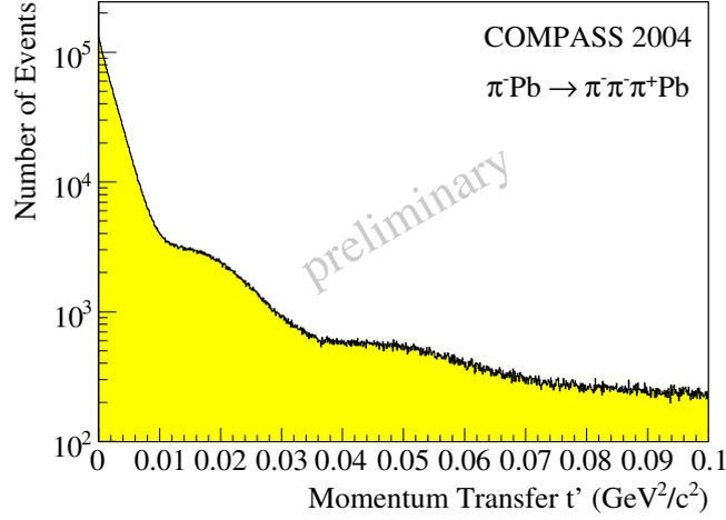
**FIGURE 3.** Measured momentum transfer spectrum in the reaction  $\pi^- \text{Pb} \rightarrow \text{Pb} \pi^- \pi^- \pi^+$ . The Primakoff region  $t' < 0.001 \text{ GeV}^2/c^2$  covers only the lowest bins of the distribution, the adjacent low- $t'$  region up to  $t' < 0.01 \text{ GeV}^2/c^2$  shows the characteristic  $e^{-bt'}$  behaviour of a diffractive process.
