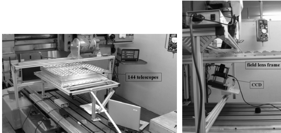
Fig. 4. Measurement of the field lens frame and whole telescopes. The milling machine setup.
