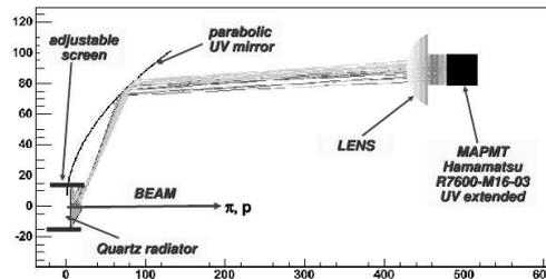
Fig. 1. Schematic view of the 2004 test beam setup.
