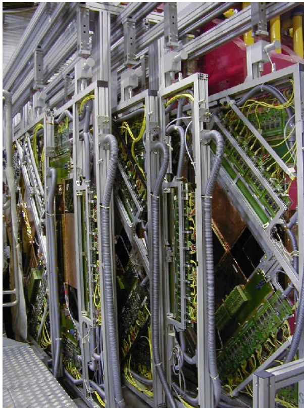
Fig. 16: The micromegas telescope installed in the COMPASS spectrometer.
