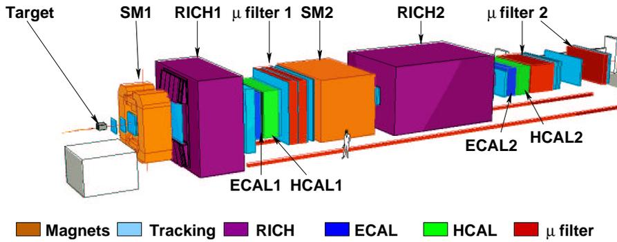
Fig. 1: General setup of the COMPASS spectrometer.
