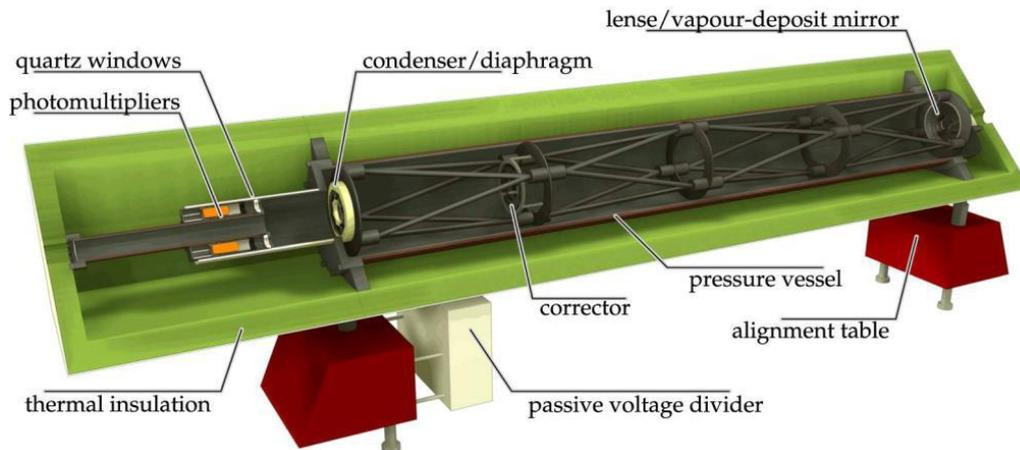
Figure 39: CEDAR 2018 upgrade for better rate- and thermal stability.
