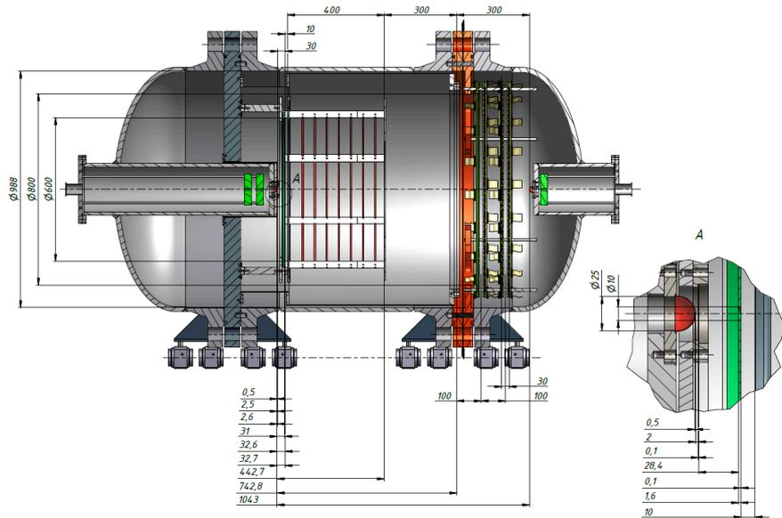
Figure 41: Sketch of the target TPC with pressure vessel as conceived for an elastic  $e^-p$  scattering experiment at MAMI. The forward tracker system on the right side of the vessel will not be installed for the M2 measurement.
