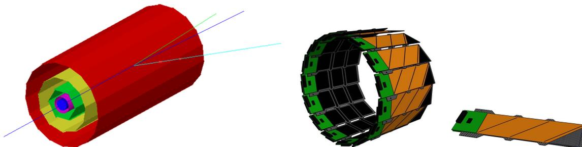
Figure 45: Left: 3-layer silicon detector (SD) surrounding the polarized target, with trajectories of particles emerging from an exclusive DVCS event: proton (light blue), photon (green), muon (blue). From inside to outside: target, MV cavity, inner SD, middle SD, outer SD. Each layer is  $300\ \mu\text{m}$  thick. Middle: conceptual design of outer SD layer with 300 mm diameter, right: SD ladder design.
