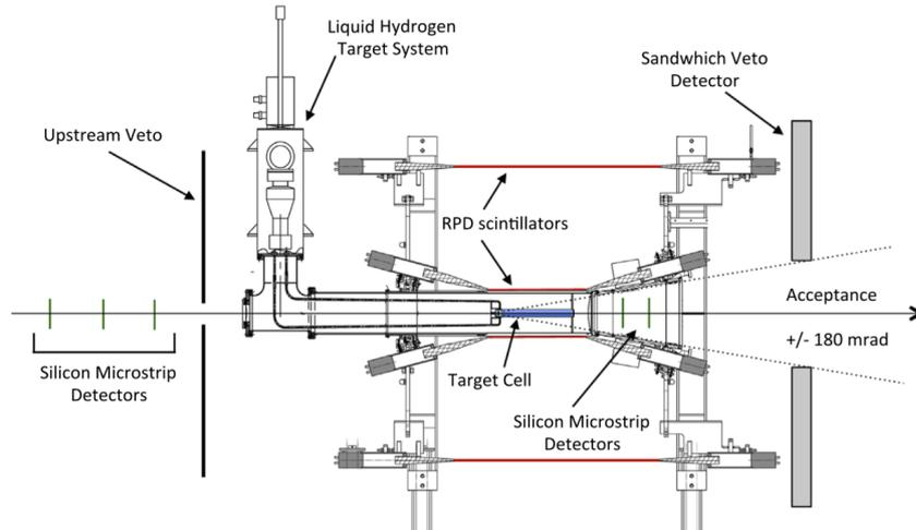
Figure 21: Longitudinal section of the COMPASS liquid  $H_2$  target.
