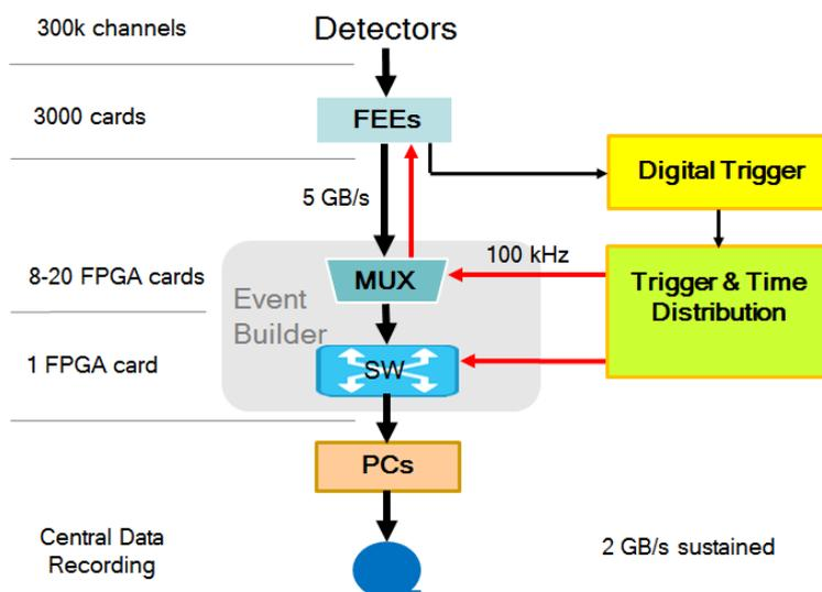
Figure 38: The DAQ architecture of the new experiment.
