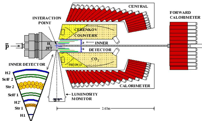
Figure 47: Schematic view of the E835 setup at Fermilab [71].
