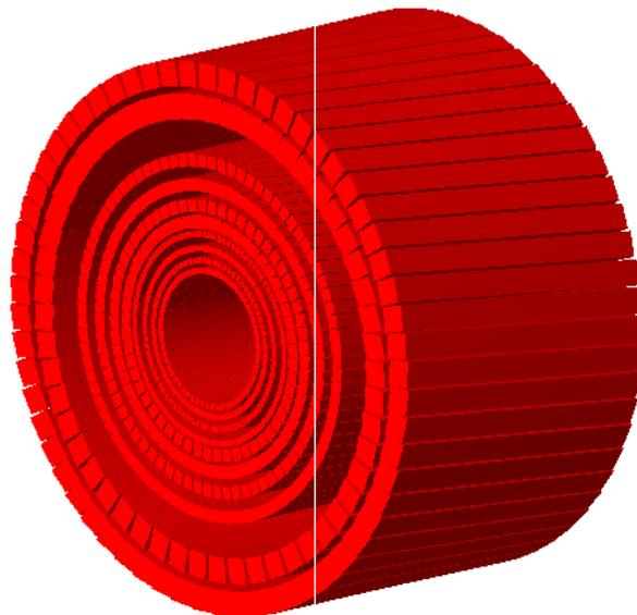
Figure 42: Layout of the recoil proton detector used for the high  $Q^2$  range.
