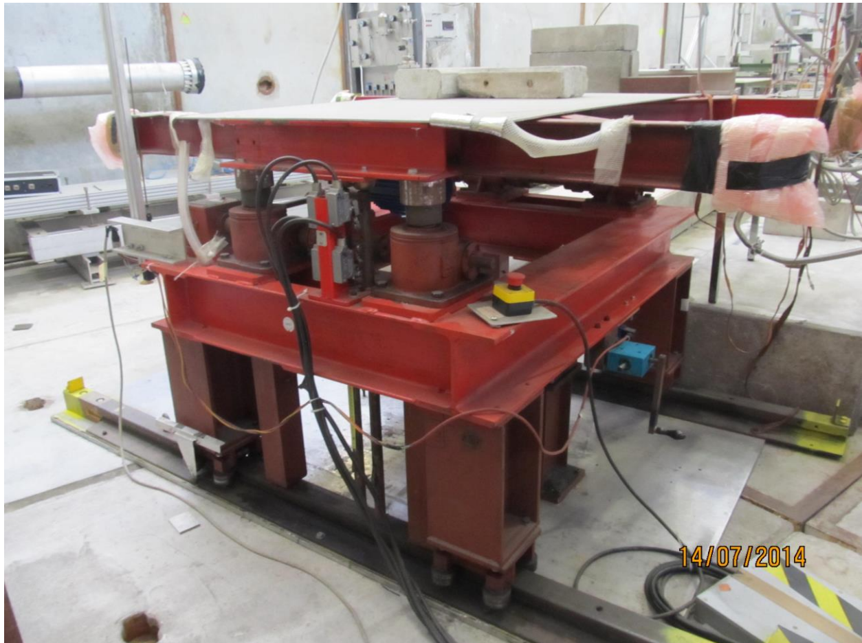
Fig.2. The moving platform is already installed at T10 and will be used as support for ECAL0 modules.
