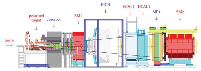
The inner part of the hadron absorber shown below consists of a tungsten rod surrounded by alumina and stainless steel. The outer part is made by concrete blocks. The whole design is checked in numerous simulations with RP.
